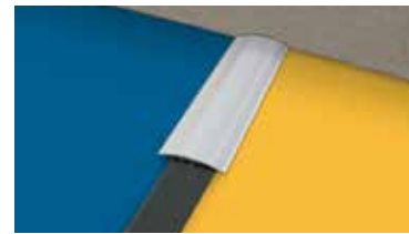
ADAPTABLE TRANSITION STRIPS Aluminum adaptable transition strip Compensating up to 14mm difference in level 1 box of 10 pcs - 27lm 41mm high x 2700mm long
