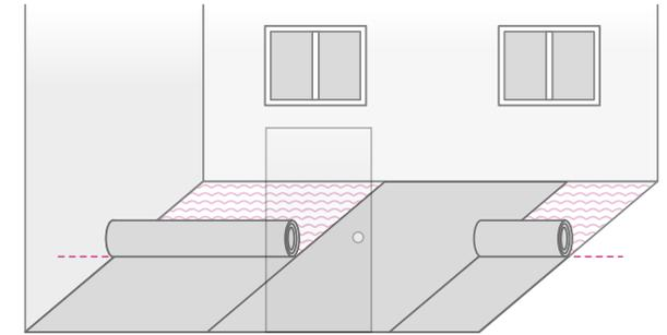
It's important to use the cork press when you gradually roll out the sheets onto the adhesive. In this way, you will avoid catching air under the sheets that may cause blisters later on.
