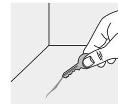
When the subfloor is not hard enough, significant traffic or heavy load could damage screed/levelling compound and could cause visual/technical defects.
